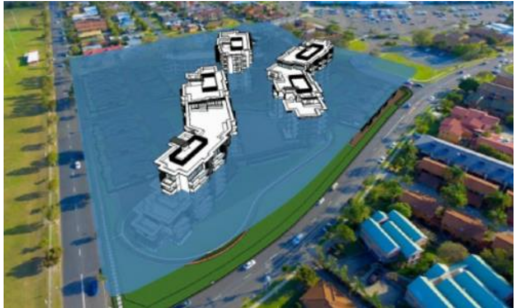
3D model of the proposed development showing the 15.5 metre height control represented by the blue coloured plane.
